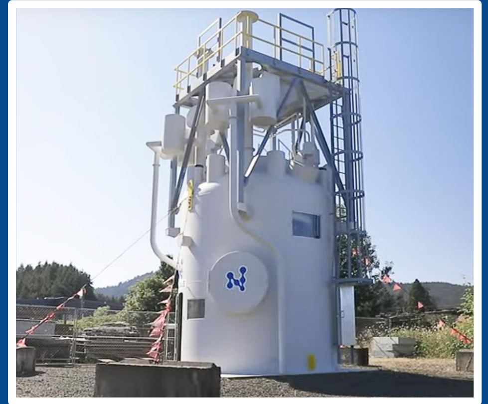
NuScale Power SMR Upper Module Mockup
